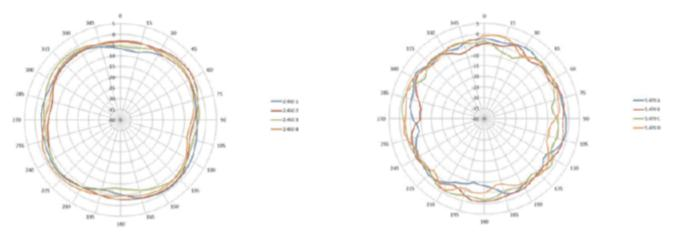
Horizontal or Azimuth plane (top view), 0 degrees downtilt 2.450 GHz 5.470 GHz
